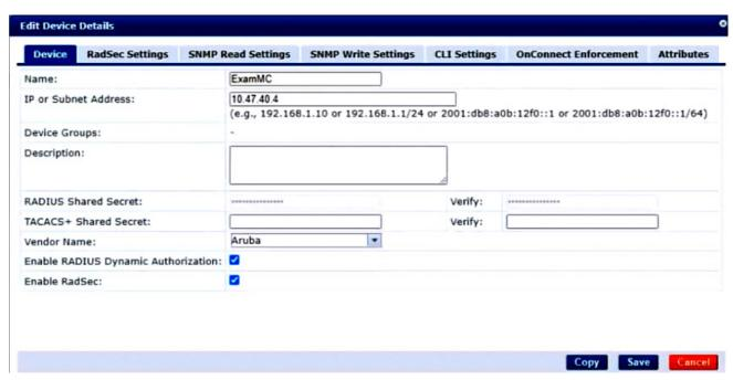
The MC is already configured with RADIUS authentication settings for CPPM, and RADIUS requests between the MC and CPPM are working. A network admin enters and commits this command to enable dynamic authorization on the MC: aaa rfc-3576-server 10.47.47.8
