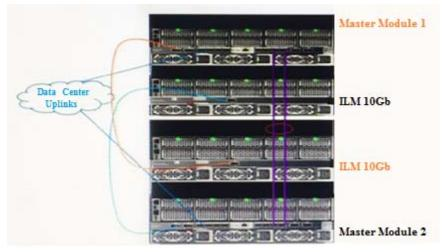
A customer with the configuration shown attempts to configure a server profile for a now application that requires 20Gb of bandwidth, but the configuration fails. The HPE SV 480 Gen9 compute modules have two Intel Xeon E5 - 2695 v4 processors. 256GB of RAM and HPE Synergy 352QC Converged Network Adapters installed.
