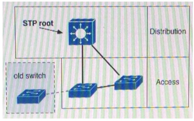
A. network engineer deployed an older switch with the same spanning-tree priority as the existing root, which caused a network outage.
